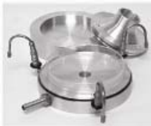
BUCK-BioAire™ Single Stage Sampler fully disassembled, showing bottom plate with Petri dish, airflow classification stage and inlet cone.
